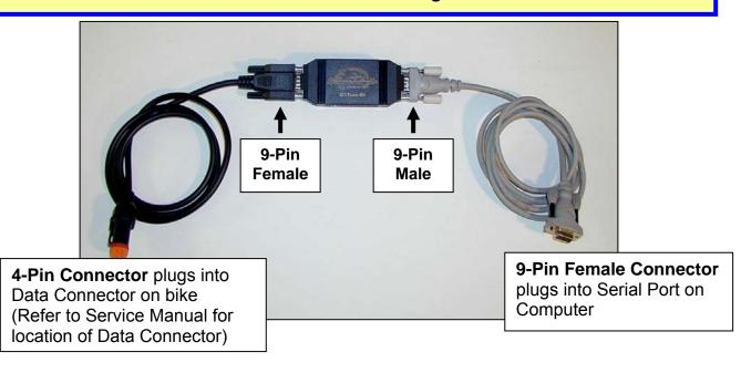
**Note**: The **EFI Tuner Interface Module is a "single unit" design** that permanently links to the ECM the first time communication is established. The Interface Module can then be used an infinite number of times with that ECM, but the Interface Module will not communicate with any other ECM's.
